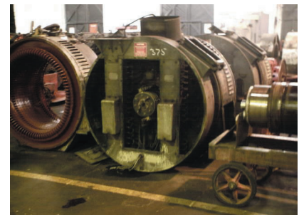
AR-10 Alternator is rotated by the diesel engine, producing electrical current to the traction motors
