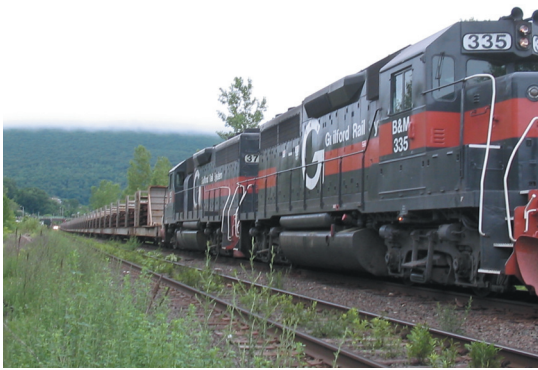
Delivering the New Welded Rail for Tunnel Distribution Photo by Phil Corder
