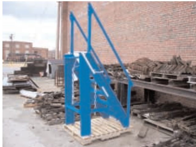
Stairs designed for entry into traction motor pit by Waterville safety committee members
