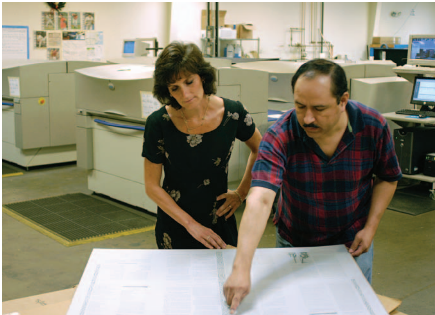
Plant Manager Christine Holmes inspects a plate with CTP Platemaker Juan Portillo. Westford's side-by-side, high-speed thermal plate imaging systems can produce 55 plates per hour—more than the presses require. Redundant capacity at the front end allows the plant to react quickly and deliver consistently.
